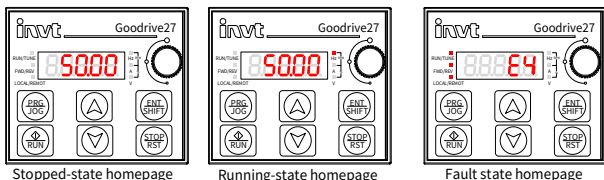
Figure 5-2 Status interface display
